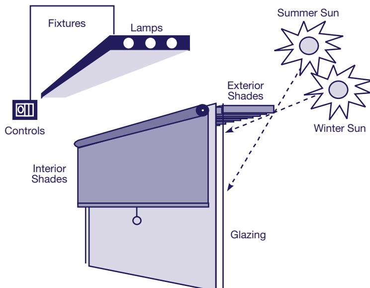
80 percent in comparison to unshaded clear glass. Air space between exterior shades and windows helps carry away heat absorbed by the shade before it can be transferred through the window.
